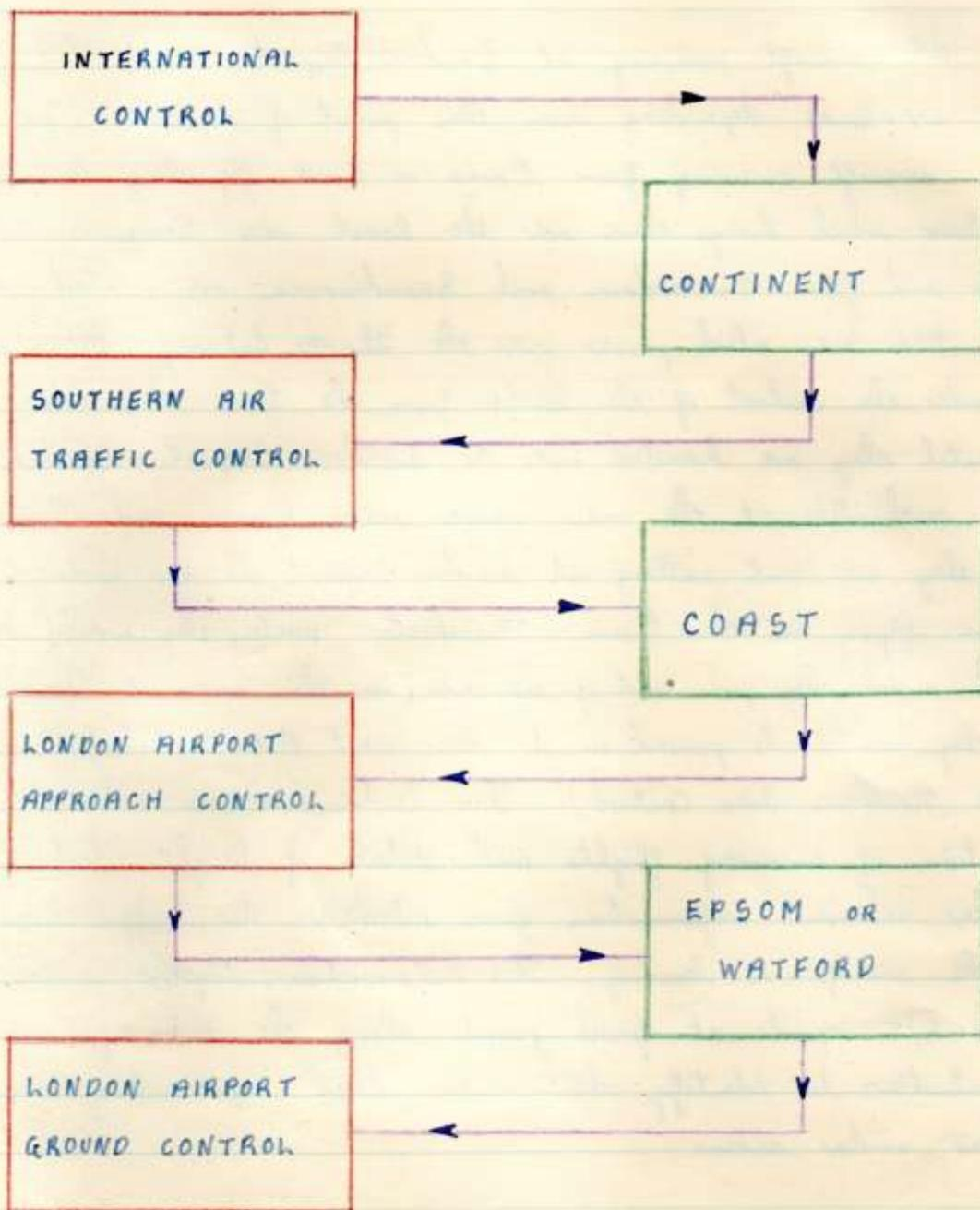
integrated in order to bring on airlines flying in on an airway from outside Britain safely down onto one of the runways of London Airport and to guide it until it has reached its own particular unloading bay.
