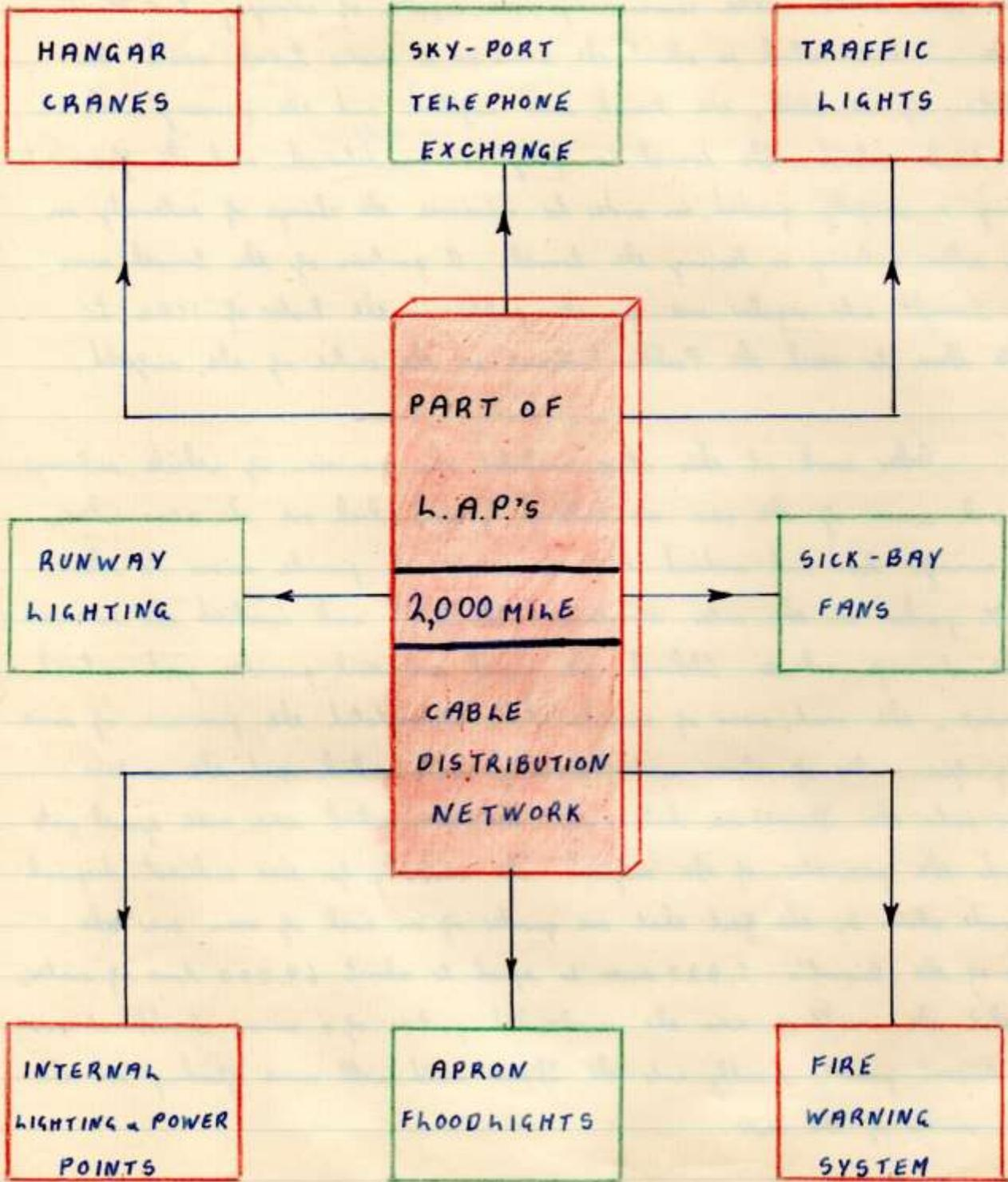
airfield. The electricity cables, over two thousand miles of them, carry the current from the forty-five sub-stations to the widest variety of electrical apparatus imaginable from giant cranes in the hangars and powerful floodlights on the marshalling apron to traffic lights in the Tunnel and electric fans in the sick bay.
